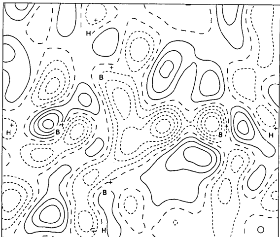
Fig. 7. Axial map through the centre of the REDCOP boron cluster, the apical B-atom positions and B(2) showing the asymmetric peak below B(1). Contours as in Fig. 2. Map dimensions 6.187 \times 5.221 \text{ \AA} .
